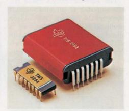
Having a capacity of 92,304 bits, it's the first commercially available magnetic bubble memory. A natural for applications where portability is desired in programmable calculators. Data loggers. Voice storage. Measurement and test equipment.
