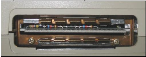
Figure 2 - Copper Bushings
